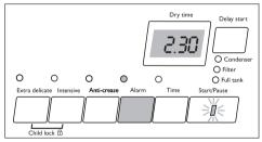
To deselect the function press the *Alarm* button again. The LED above is off.
